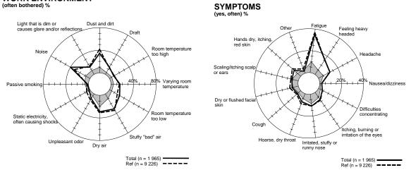
Figure 1. The perceived indoor climate and symptoms for the two databases. The shadowed areas show the reference data for workplaces without known indoor climate problems (Andersson et al., 1998).
